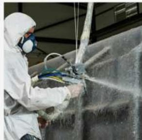
6. Fibreglass and resin spraying
